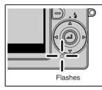
Flashes while the camera is accessing the memory card, such as recording images to memory card or reading data. While the LED is flashing, do not open the card/battery cover or remove the memory card.
